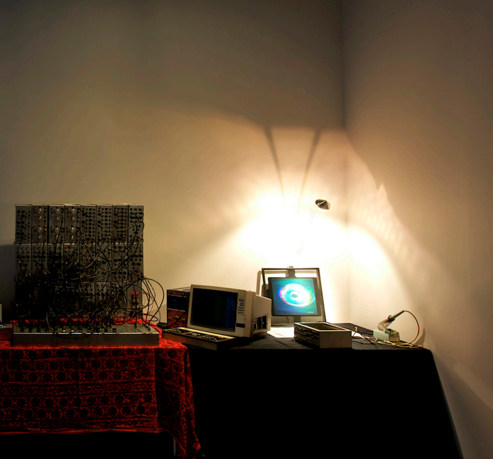
ON TABLE: SANDIN ANALOG IMAGE PROCESSOR. THIS VIDEO SYNTHESIZER WAS USED STAND-ALONE OR IN CONJUNCTION WITH GRASS SYSTEM FOR MOST VIDEOS IN THE SHOW. PHOTO BY JOHN HANACEK
